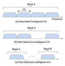
Figure 1. The illustration of carrier aggregation (CA) [5]
